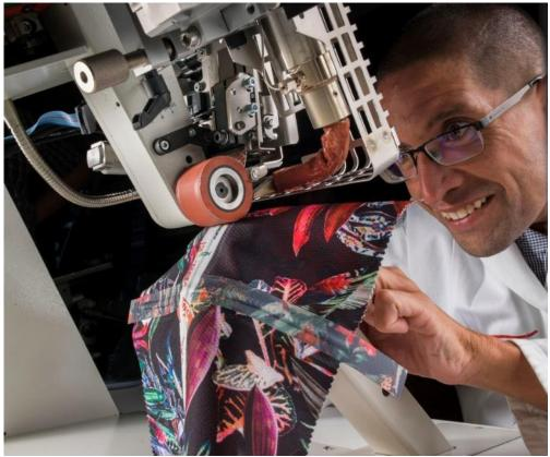
To match the laminate design, Trans-Textil prints its new Topaz Elements® Tapes using the environmentally friendly digital transfer printing process.
